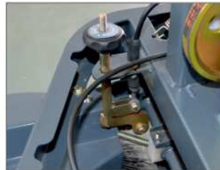
Easy access to broom adjustment system
