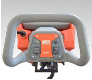
All operational switches are within direct view and easy reach of the operator. Excellent view of the area of be cleaned.
