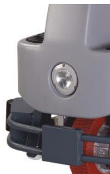
Centrally placed wide angle head lamp for good visibility while operating in low lit areas.
