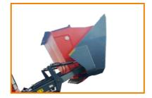
The large hopper with 900L capacity supports longer operations.
