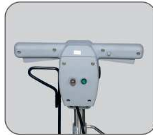
The handle is equipped with safety switches.
